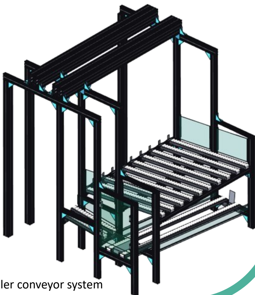
Figure 4: Roller conveyor system
