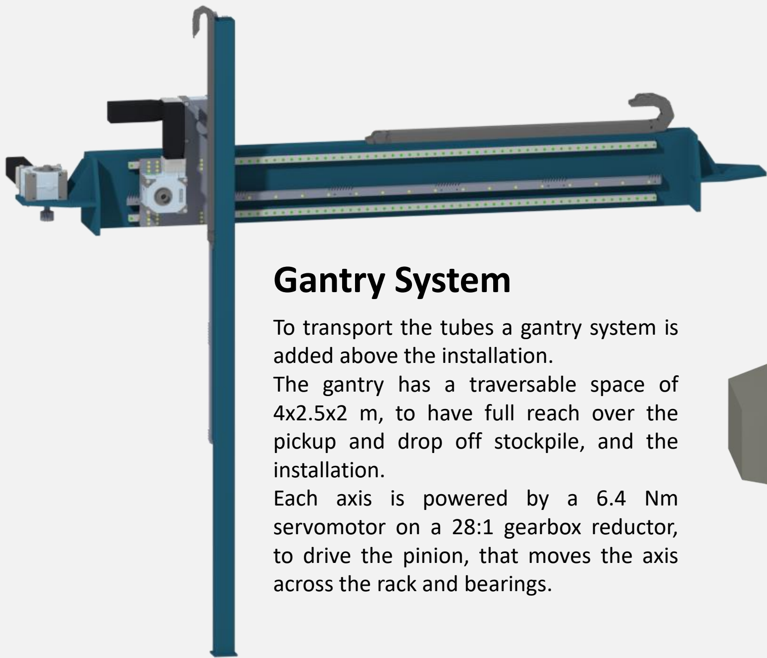
Figure 3: YZ axis of Gantry system
