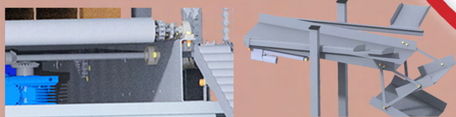
Figure 9: Inside view in palox discharge conveyor Figure 10: Apple filling system for a soft landing
