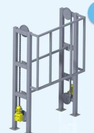
To solve the problem of storing the cloths, a buffer was created that can automatically rotate the total of 19 rolls. This allows quick selection of the right roll to cut the required cloth size. The buffer is capable of carrying and rotating 19 rolls, each weighing 435 kg. In addition, the buffer can easily load new rolls and unload empty rolls from the rear. To ultimately ensure safety for the operators and the environment, fall protection and sturdy materials are used.
