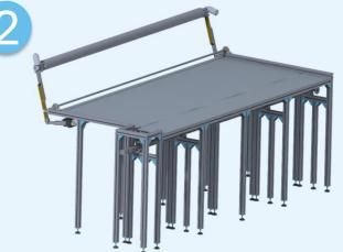
Also present on this table is a motorized rail, which holds a carriage. Mounted on this carriage is a cutting disc attached to a motor. The disc protrudes slightly from the table surface to be able to cut the cloths with high precision.
