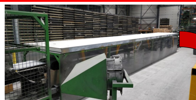
Figure 3: Step 9 heating tunnel
