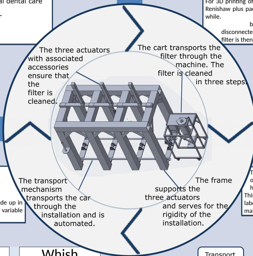
The goals of the project is to design a transport + cleaning installation that makes it possible to efficiently and ergonomically clean the filters of 3D printers.
